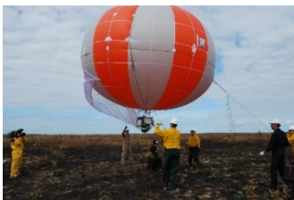
Researchers prepare to launch a balloon into a smoke plume to measure emissions during an operational scale fire. USDA Forest Service.
