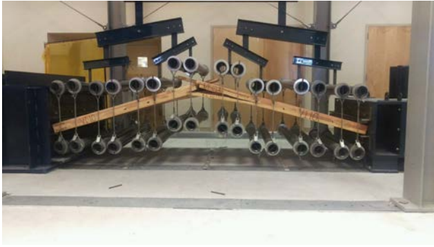
Load tree testing of cross-laminated timber (CLT) panels at Tyndall Air Force Base.
